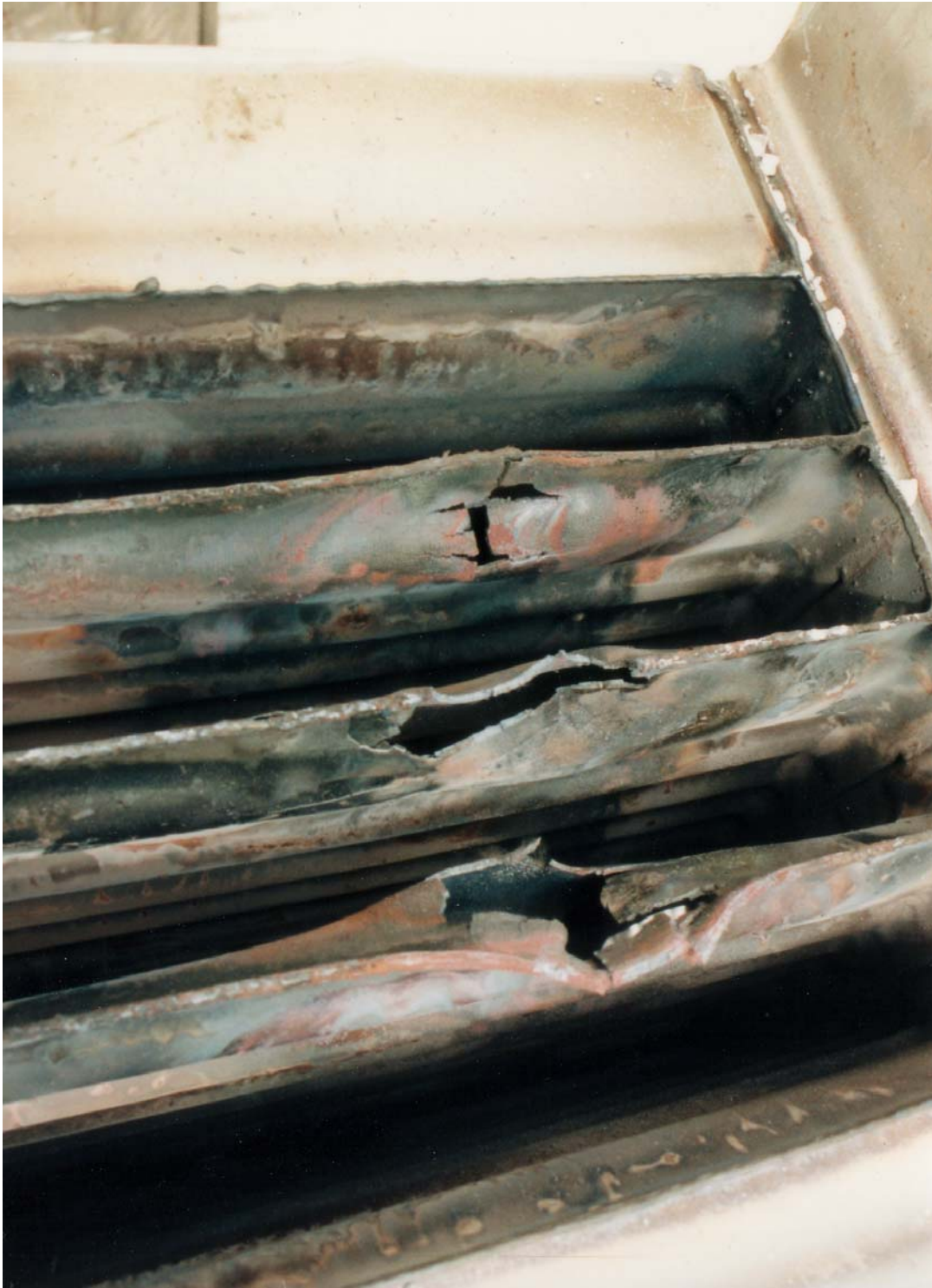
Photo Six: Failed heat exchanger.
